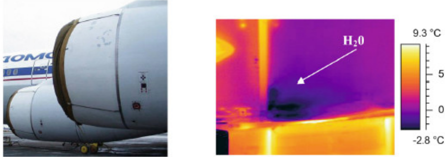
Figure 4.2: Passive IRT thermographic diagnostics of water ingress in the honeycomb aluminum air inlet of an Ilyushin-96 airplane
